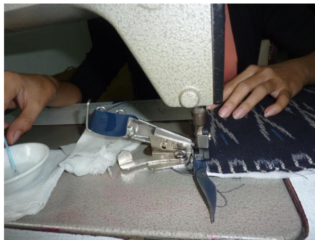
This tool was created to mechanically glue the border of the cover
